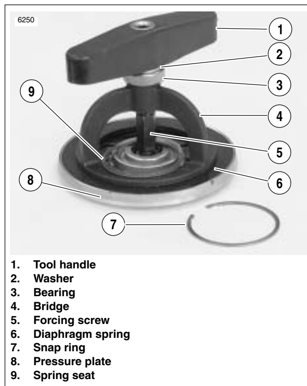
Figure 6-14. Pressure Plate Assembly
